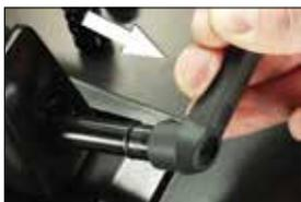
The tension on the lock lever may be adjusted by pulling the handle away from the mount. This disengages the handle from the screw mechanism and allows the lever to be reoriented.
