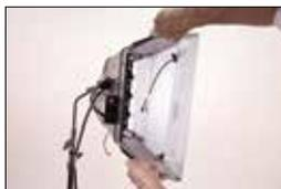
Expand the Barndoors to smooth out the face of the Flozier and eliminate wrinkles.
