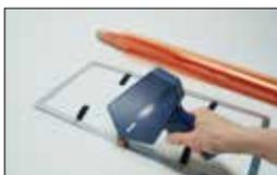
Rotate all Velcro tabs to the inside of frame. Apply double sided transfer tape to one side of the gel frame.
