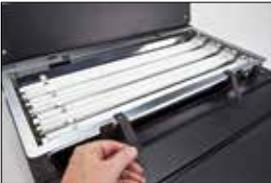
The Gel Frame is held to the fixture with 4 Velcro straps.
