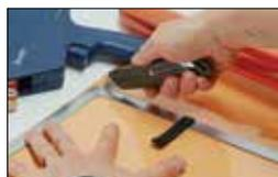
Trim the excess gel from the frame. Rotate Velcro tabs back into position.
