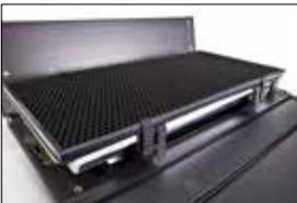
The Louver is fastened to the fixture with 4 Velcro straps.
