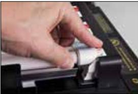
To remove, press red locking tab down and pull up on lamp.
