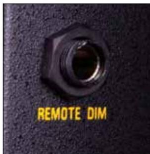
Insert the dimmer cable into the receptacle marked **REMOTE DIM**.
