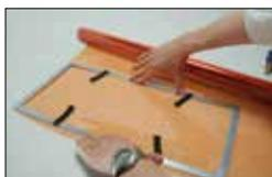
Lay the taped side down on the gel and press firmly for adhesive to adhere.
