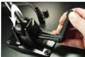
A 180 degree turn loosens the orientation of the mount. A right turn tightens the mount.
