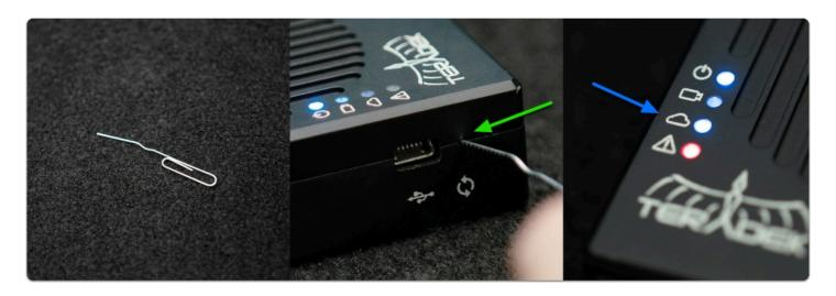
Select 'PAIR' on the 703 Bolt and the monitor will begin pairing which typically takes 5-10 seconds but can take up to 3 minutes in the presence of heavy 5Ghz interference.
