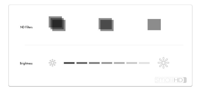
Lens filters offer creative flexibility on brightly lit scenes - instead of having to raise shutter speed and increase strobing, or close down the aperture and deepen the depth of field, ND (neutral density - aka darkening) filters can darken the shot without adjusting the aesthetic.
