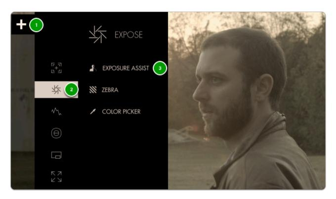
Once added you can **edit** the settings by **navigating right** or tapping the right arrow when 'Exposure assist' is highlighted.
