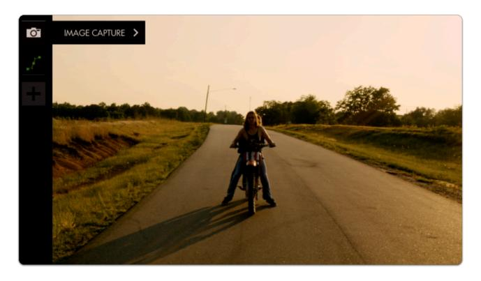
A grey snapshot overlay will appear; click the joystick or tap the screen and the overlay turns green, indicating a snapshot has been taken.
