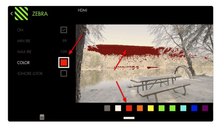
At this stage we can roll **exposure down**, add an **ND filter**, **decrease ISO** or **increase shutter speed** to **darken** the image until the zebra pattern is no longer visible to get **highlight detail back**.
