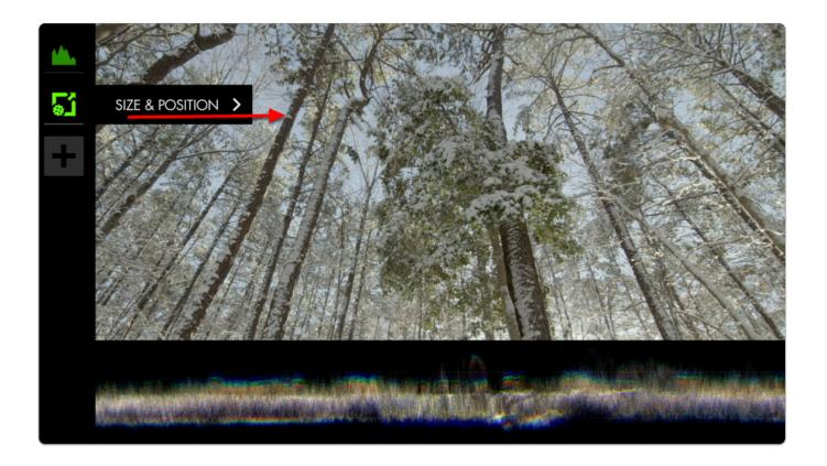
Navigate to SIZE and adjust it from 100 to 75- you will notice the image scaling from its' center point.
