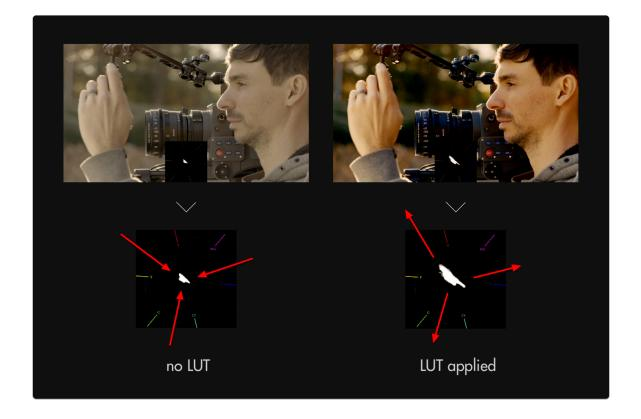
The Vectorscope uses the same layout as a **color wheel** and therefore principles of **color theory** apply - for example we can achieve **complimentary** colors by ensuring our scene plots to the graph on **exactly opposing sides**. Perhaps the most common example of this is the famous/infamous 'teal/orange' look popularized in Hollywood where skin is orange and nearly everything else gets colorized as teal.
