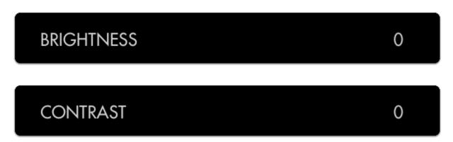
Adjust the brightness/contrast of the image to feed the Peaking filter with an adequate (ie not a flat log signal) source, translating into a clearer view of what is in focus.
