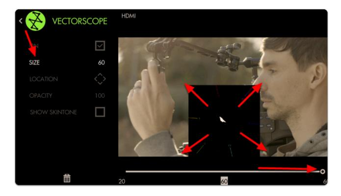
You can adjust the **SIZE** of the graph for better visibility. At this stage feel free to use **Size & Position** or **Crop & Scale** to **arrange** the image and scope so that they **don't overlap**.
