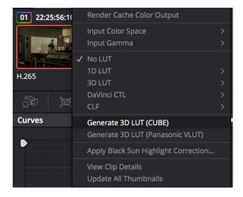
9. Save to an SD card for use in SmallHD monitors and elsewhere (ensure that the file retains a .cube extension or the LUT will not be recognized by the monitor).
