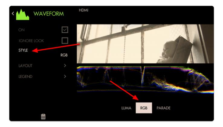
Back out of the Edit Tool menu to observe the waveform in action and to accurately expose your footage.
