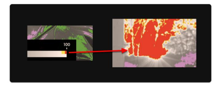
Clipped areas are tricky to manipulate in post production because they are effectively comprised of a single 'blob' of color/value.
