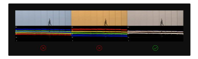
Notice how adjusting the white balance setting on the camera shifts the RGB 'bands' - when lined up they **turn white**, indicating a **proper white balance** setting.
