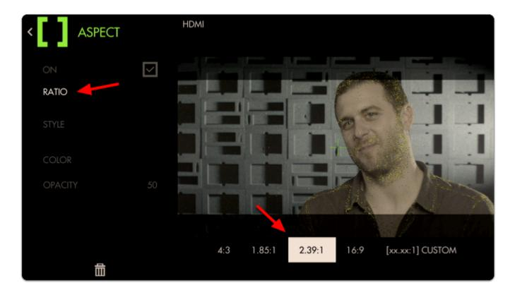
Navigate to "Ratio", select it and change the aspect ratio to "2.39" for cinemascope viewing.
