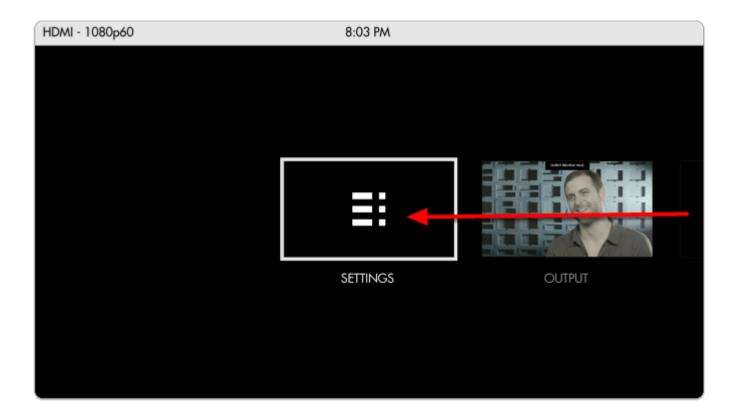
To select the monitor's input **press the joystick left** until you reach the **Monitor Settings** page. Navigate with the joystick to the (1) **Input section** and click to go 'into' the input menu. From here (2) **select HDMI or HD-SDI** depending on which signal you wish to display.
