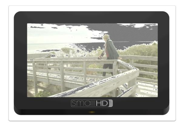
Zebra is essentially a simplified version of Exposure Assist which allows the specific 'painting' of areas depending on brightness value but is less destructive to the underlying image — it is however limited to painting one value range at a time, though up to two Zebra tools can be activated simultaneously. Click to learn more about the Zebra tool.
