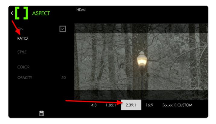
By default the bars are set to 50% opacity; adjust 'style' and 'opacity' to taste for whatever you find most viewable. Here I set the opacity to 80% to keep the off-screen areas from being distracting.
