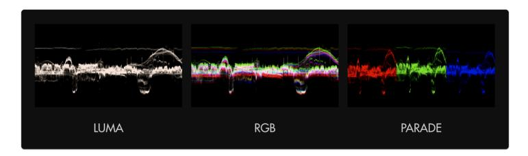
Pick your flavor of Waveform- LUMA displays a brightness/luma plot only while RGB graphs each primary color on top of one another. RGB PARADE physically separates the Red, Blue and Green channels into discrete sections from left to right so they can be viewed easily in isolation.
