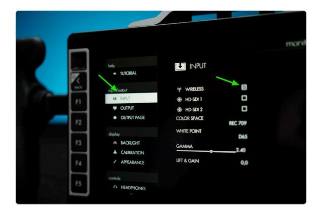
Press the Back button & navigate downward to find the **WIRELESS** option under the **ACCESSORIES** category.
