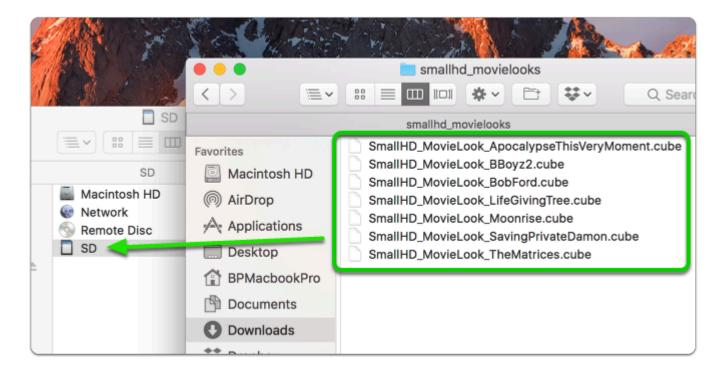
With the LUTs placed on the SD card, insert it into your monitor. From any page with a video feed, click the joystick or tap the screen to bring up 'Add New Tool' and navigate to Overlay > Look.
