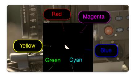
If we **apply a <u>LUT</u>** to this page, the Vectorscope reacts by **expanding** its plotted area. The scope confirms that we are viewing a more heavily saturated image after applying the look.
