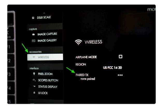
Click the joystick and select **PAIRED TX** to enter pairing mode which will wait for a wireless signal from a <u>compatible transmitter</u>.
