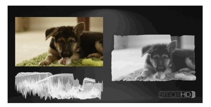
The **Waveform** is generally considered the **most robust exposure tool** because it plots your image's luminance (brightness) -- and chrominance if using <u>RGB mode</u> -- to a graph but unlike the Histogram, it physically **matches the screen from left-to-right**.
