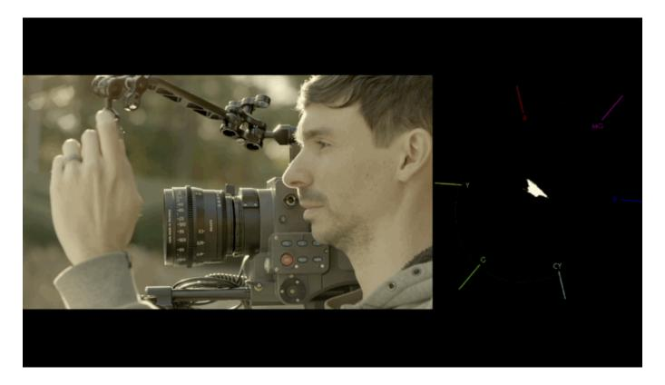
Though generally not considered as 'mission critical' during shooting as exposure scopes such as Waveform & Histogram, the **Vectorscope** plots the **chromacity**, or the **hue + saturation** of your image onto a **color wheel** so you can help gauge **complimentary color**, ensure **skin tones** are being colorized properly, to visualize how overall scene color is being placed, and where potential adjustments may need to be made in general.
