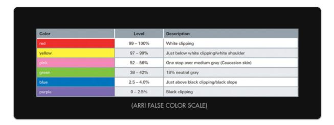
This allows you to make exposure decisions that are based on **numeric values** as opposed to simply how the image **appears**, which depending on viewing environment and many other factors can yield inconsistent results.
