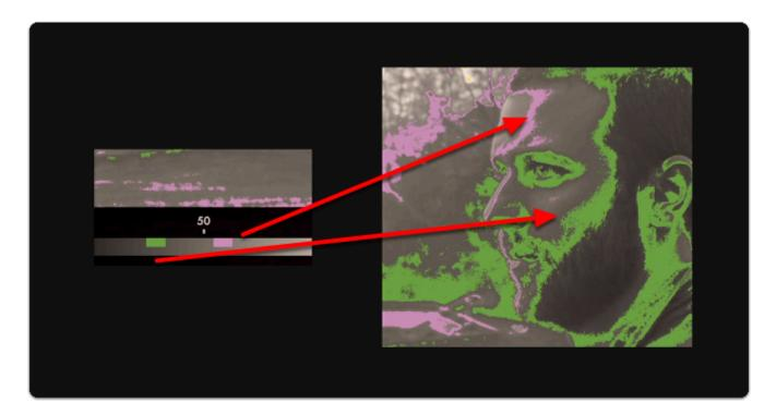
Sticking with this exposure value means we'll be **clipping** a portion of the sky & sun - Exposure Assist makes it clear which areas will be clipping/losing detail as a result of overexposure by painting such areas **red**.
