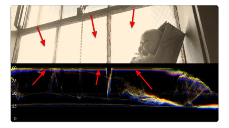
**Rolling exposure downwards**, the lines 'un-flatten' and much more of the window can now be manipulated in color grading while some areas remain overexposed.
