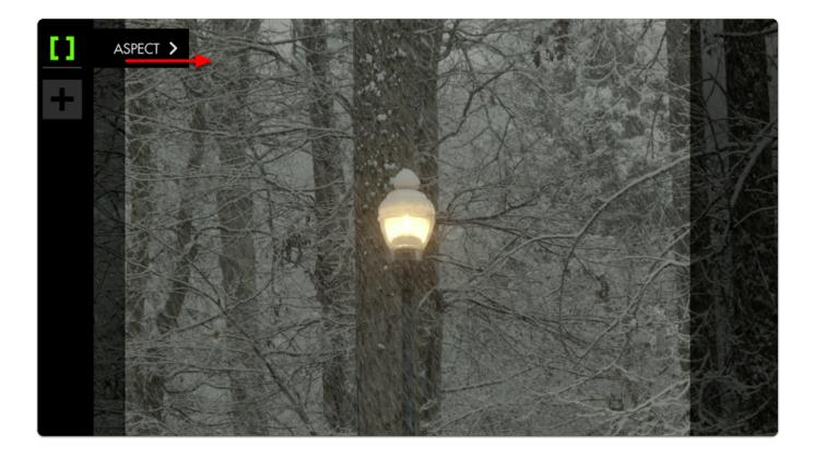
The **default** setting is for previewing a **4:3** aspect ratio for older TVs. Select 'Ratio' and change it to **2:39** to see the black bars switch to a horizontal configuration.
