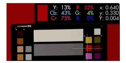
**Color Picker** samples color/value information from a **single pixel** to give a precise readout of a specific location. Great for **matching** multiple cameras or getting **consistent exposure** in changeable lighting conditions by sampling from a color chart or an actor/subject's face.
