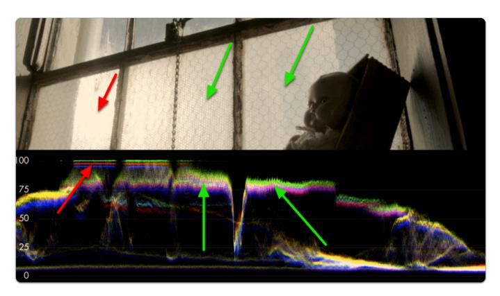
If we keep rolling exposure down (closing the aperture) we will continue seeing more 'into' the brighter details at the expense of **shadow details** which become 'crushed' or 'clipped' and effectively lost similar to overexposure.
