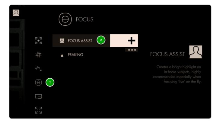
**Focus Assist** will paint a **highlight** around areas it determines to be in focus based on small/harsh changes in contrast.
