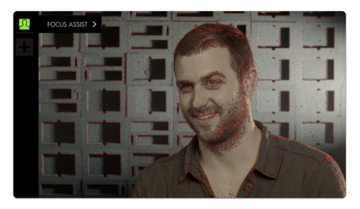
To fix this, **edit Focus Assist** by **pressing to the right** when it is highlighted in the tool bar, and navigate to **Peak Threshold**.
