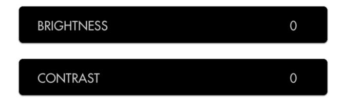
Adjust the brightness/contrast of the image to feed Focus Assist with an adequate (ie not a flat log signal) source, translating into a clearer view of what is in focus.
