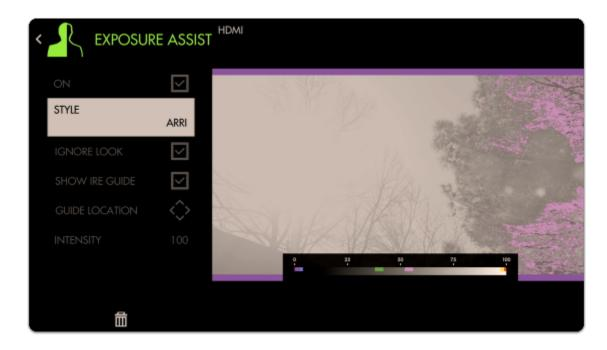
Even though the sun area is clearly clipping, the Arri false color scale doesn't pick it up - we need to fix this for an accurate reading.
