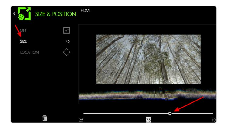
Now move the image to the top of the frame by selecting **LOCATION** and pressing **up on the joystick** or **tapping the top portion of the image**. This leaves us with an unobstructed view of the **Waveform**.
