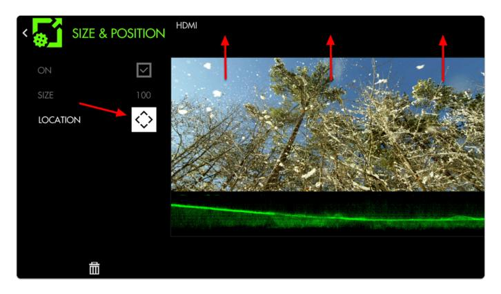
Back out of the edit menu for a **full-screen** view of a **2.39 cinemascope aspect ratio** accompanied by a **full-width** <u>Waveform!</u>
