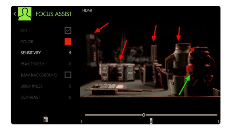
Notice how we are picking up many edges that are **not in focus** in addition to the areas that are in focus.
