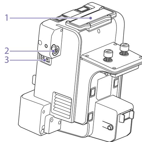
1. **Wireless receiver insertion slot**
