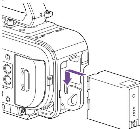
To remove a battery pack, press and hold the BATT RELEASE button (page 8), slide the battery pack up and then pull it out of the attachment.
