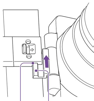
Guide groove Protrusion
