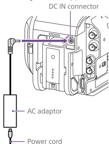
Connect the AC adaptor to the DC IN connector on the camcorder, and connect the power cord (supplied) to an AC power source.
