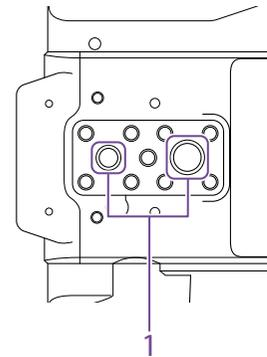
1. Tripod screw holes (1/4 inch, 3/8 inch)
