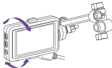
You can adjust the angle so that the viewfinder is facing the subject. Setting the MIRROR switch to the B/T position flips the left and right sides of the image on the LCD screen, but the image is recorded in the correct orientation.
