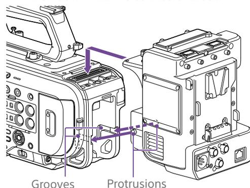
4 Tighten the two screws on the top of the XDCA-FX9 to secure the XDCA-FX9.
