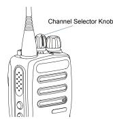
Use the Channel Selector Knob to switch between an analog or a digital channel.
