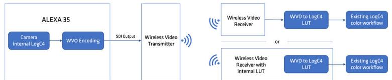
The result of the decoding LUT is a regular LogC4 signal that can be treated in exactly the same way as having transmitted LogC4 to begin with.
