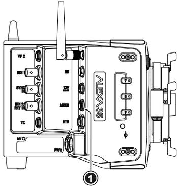
The AUDIO connector (1) is located on the right side of the camera. It is a two channel +24 dBu line level audio input with additional 12 V power output to supply microphone preamplifiers. This is the same 6-pin connector used on the ALEXA Mini LF. Use the ALEXA Mini LF Audio connector with cable (K2.0023988) to connect audio sources.
