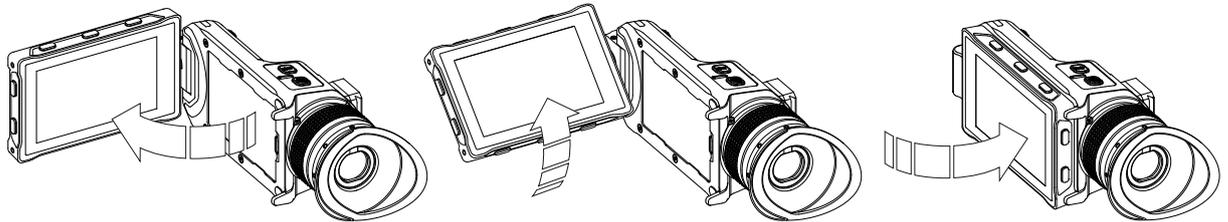
Fold out, swivel and fold in the monitor to put the display visible in the folded-in position. The image on the monitor automatically adjusts its orientation, or can be set to the desired orientation in the camera menu.
