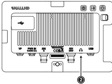
The headphones out (2) on the CCM-1 is a 3.5 mm TRS connector (headphone jack) which outputs all four audio channels with a maximum power of 2.5 dBm. The camera's headphone routing allows configuring which channels are output on the connector.
