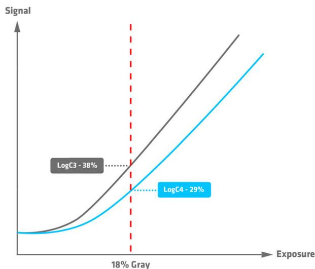
When you look at a LogC4 image, 18% gray will look darker than it used to in LogC3. Since the curve extends farther to the right in the graphic, the point of 18% gray ends up being lower on the curve.
