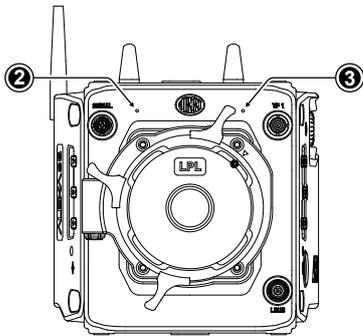
The dual gain internal microphones (2 = Internal Mic R, 3 = Internal Mic L, seen from operator point of view) are located at the camera front and can be used to record a reference track, sometimes called a "scratch track". Some software tools can synchronize the master sound with the image by using the reference track. The gain of the internal microphones is fixed, with the left microphone (3) having a gain of +18 dB and the right microphone (2) a gain of 0 dB, to cover a wide audio level range.
