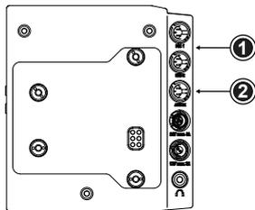
The additionally available Audio Extension Module AEM-1 supports the use of either two balanced Mic/Line inputs (1) with switchable +48 V phantom power, or one AES3 input (2). It is docked directly to the rear interface of the camera. For more information please refer to the user manual of the module.
