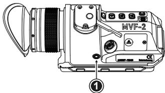
The headphones out (1) on the MVF-2 is a 3.5 mm TRS connector (headphone jack) which outputs all four audio channels with a maximum power of 2.5 dBm. The camera's headphone routing allows configuring which channels are output on the connector.
