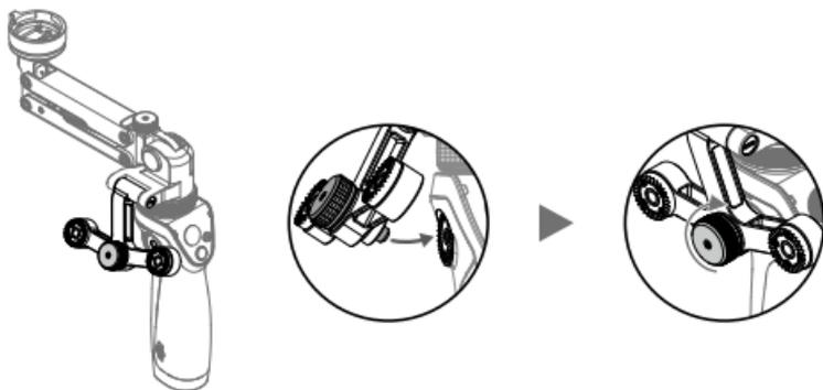
5. Rotate the Z-Axis's gimbal securing ring to its unlocked position and attach the Zenmuse X3.
